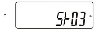
Frequency Window is +/-3 Hz. Selectable to ± 1Hz.
