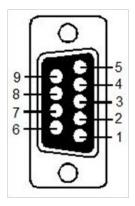
Pin 3: RS-232 Rx Pin 2: RS-232 Tx Pin 5: Ground
