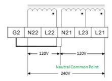
**Option 2:** 120V full capacity output. Please note the jumpers between G2-N22, N22-N21, and L22-L21 for this option. See below.
