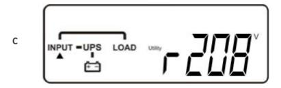
• The UPS is in self-test mode again. The LCD display will change from figure C to figure D, and the UPS will remain in battery mode for approximately four seconds. Then the display will change from figure E1 to figure F if the self-test was successful.
