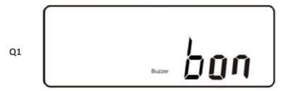
Buzzer "On". Use the 4 key to toggle the setting and then save.
