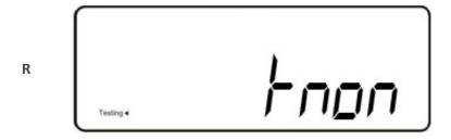
Self-test is not "On". Use the 4 key to toggle the setting and then save.
