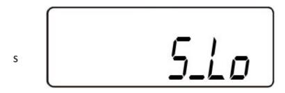
Bypass Voltage is adjusted to narrow range. Selectable to Lo or Hi.
